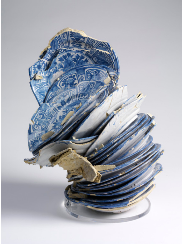
Figure 2 - Kiln Waster, Delft, Holland, 1640-1660. Tin-glazed earthenware with fragments of fire-resistant clay. Museum no. C.10-2005. A pile of 34 blue-and-white decorated earthenware plates in Chinese 'transitional style' which have collapsed during firing, causing them to deform and fuse together. Attached to it are fragments of the fire-clay kiln-furniture which supported the plates for firing
